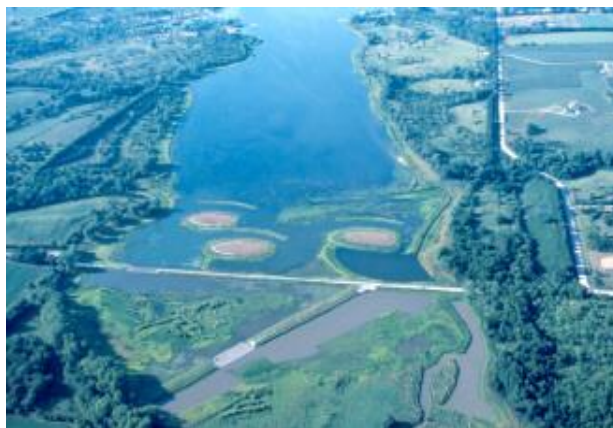
Two-Stage Sediment/Nutrient Dike and Basin
