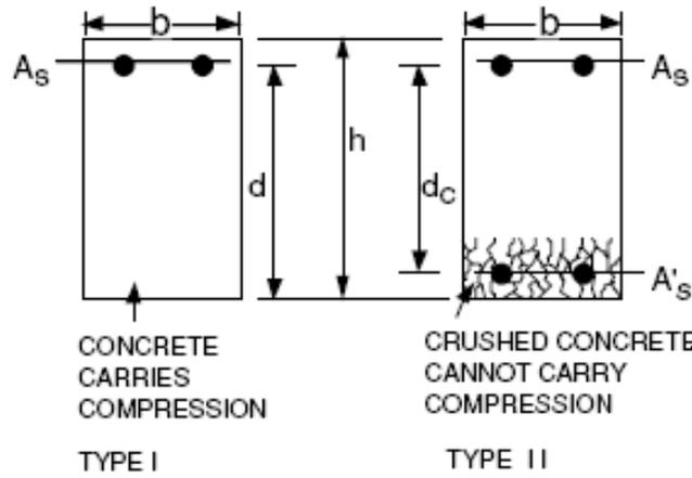
**Figure 29. Type I and Type II Cross Sections**
