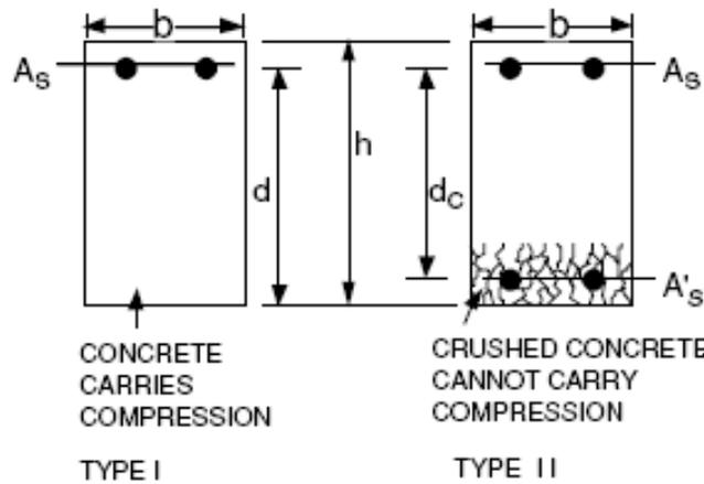
**Figure 21. Type I and Type II Cross Sections**
