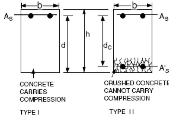
**Figure 15. Type I and Type II Cross Sections**
