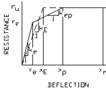
Figure 1. Resistance-Deflection Curve Showing Equivalent Elastic Deflection ( $x_e$ )
