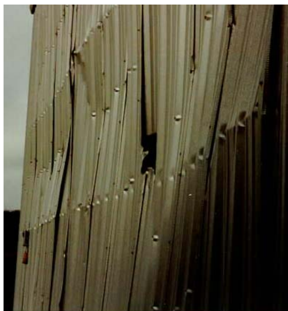
Figure 6-3 Local Buckling in Maximum Moment Region of Cold-Formed Beams and Panels
