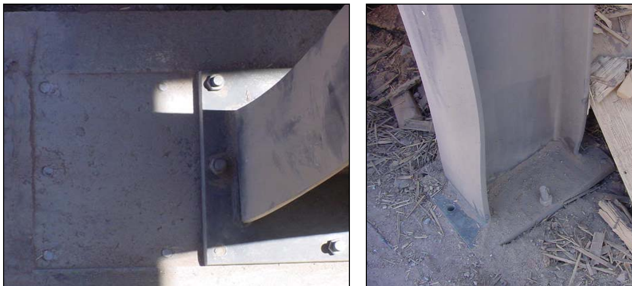
Figure 47. Failed Steel Column Connections in DB Tests
