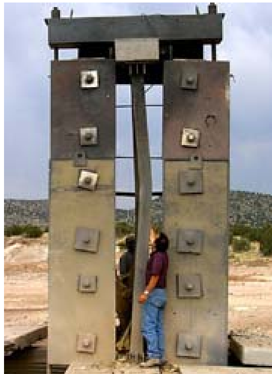
Figure 49. W14x38 Column After Blast Test
