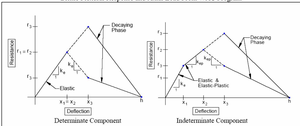
The tension membrane resistance function for steel members and compression and tension membrane resistance function for reinforced concrete and masonry members follow the methodology of UFC 3-340-01. The steel resistance function is illustrated in Figure 4 for a component with flexural and tension membrane response. The tension membrane response after yield is based on the lesser of an input in-plane
