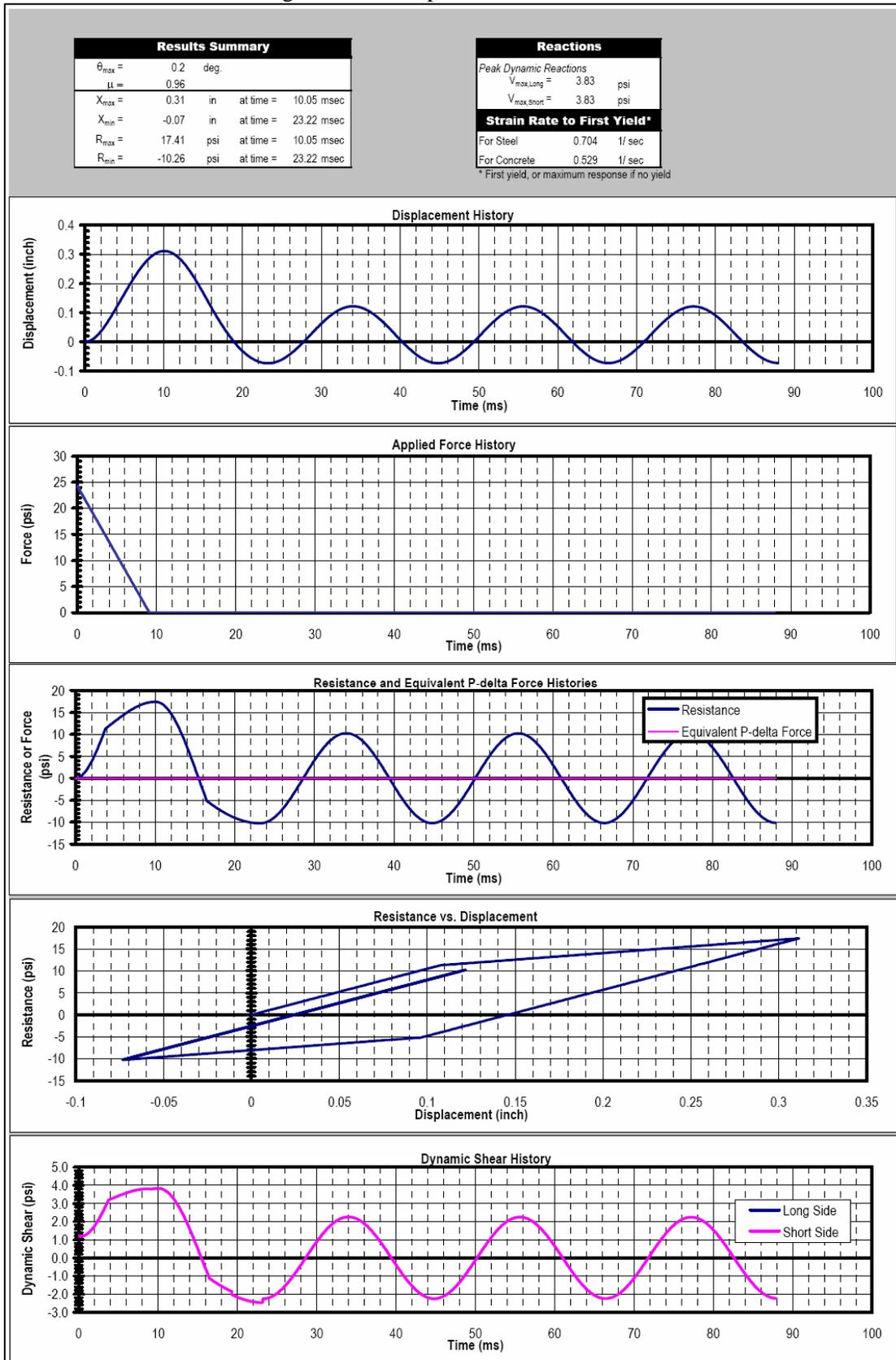
Figure 11. Example of Results Summary for Reinforced Concrete Slab
