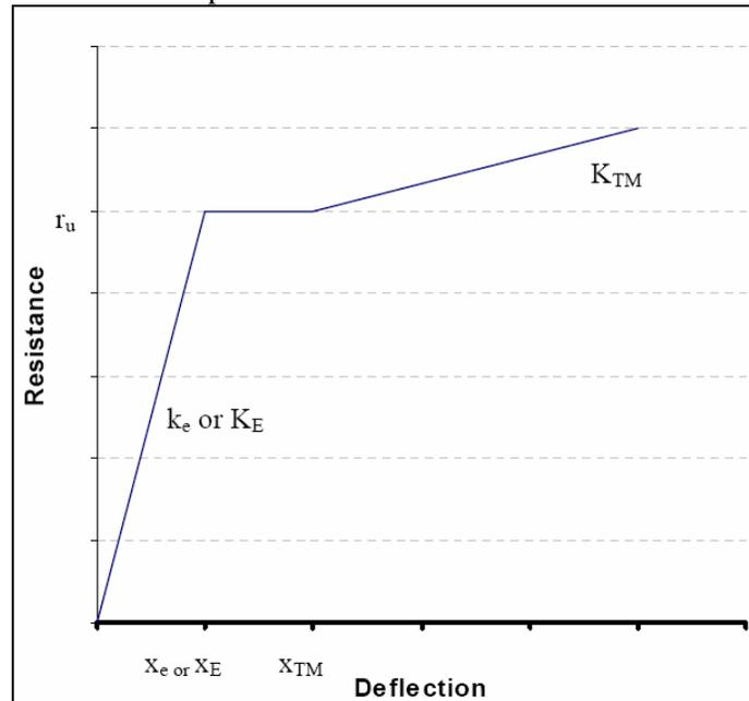
Figure 5. Resistance-Deflection Curve for Reinforced Concrete and Masonry Components with Compression and Tension Membrane (from UFC 3-340-01)
