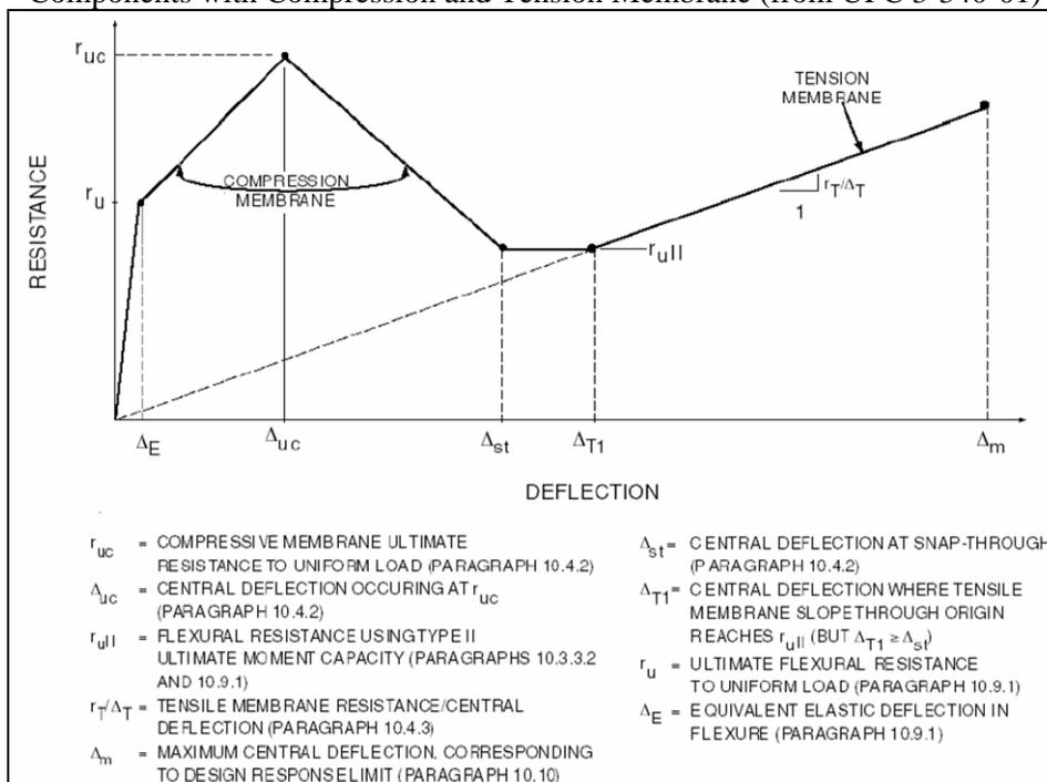
For arching of unreinforced masonry, the equations for compression membrane from Park and Gamble, “Reinforced Concrete Slabs”, were modified to allow for a gap between wall and rigid support for non-solid components, such as ungrouted CMU. The resulting resistance function is shown in Figure 6.
