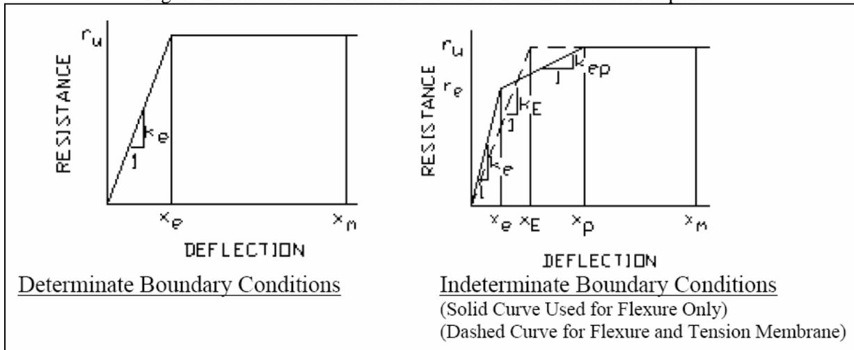
Figure 3. Resistance-Deflection Curves for Unreinforced Masonry with Brittle Flexural Response and Axial Load From WAC Program
