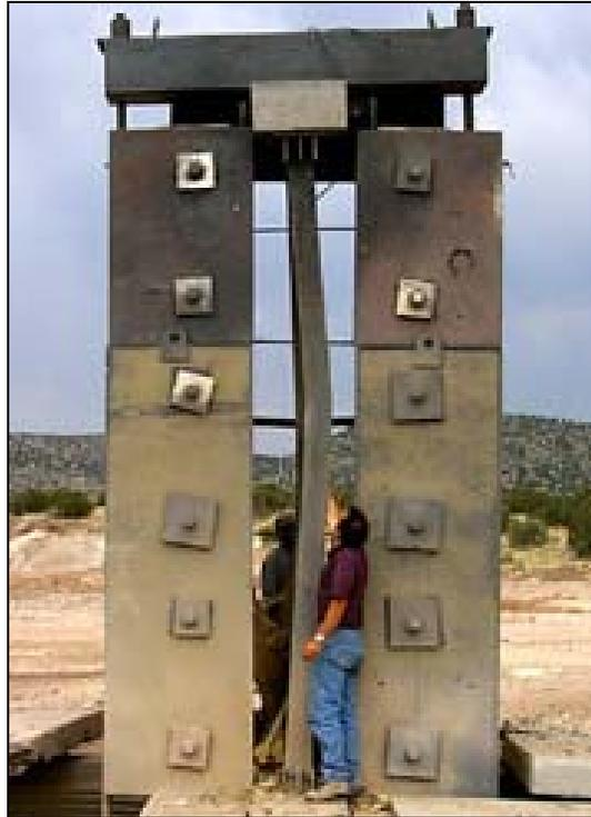
**Figure 54. W14x38 Column After Blast Test**
