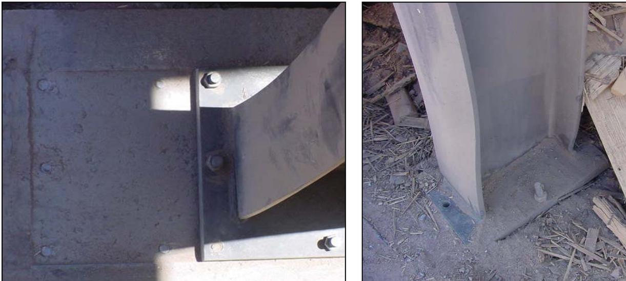
**Figure 50. Failed Steel Column Connections in DB Tests**
